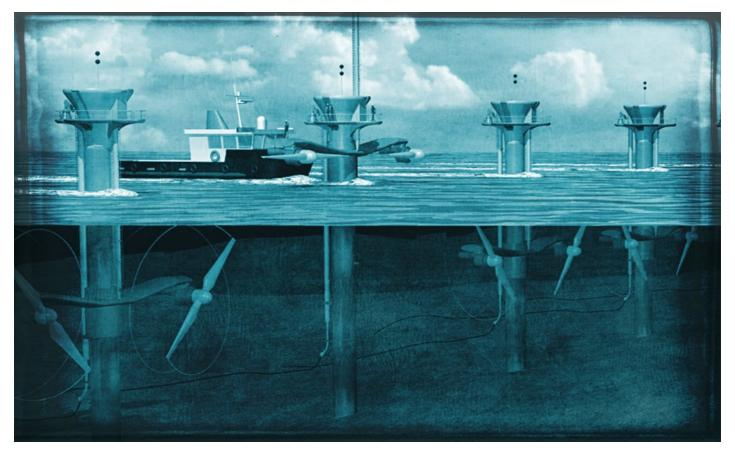
Tidal turbines are like "underwater windmills" except the rotors are driven by consistent, fast-moving currents. The submerged rotors harness the power of the marine currents to drive generators, which in turn produce electricity.
