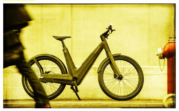
The solar bike is a self-sufficient E-Bike with fully integrated solar panels for charging. A solar film is the functional design element which is used to charge the battery. The bike is also charging while riding and when it is not in use.
