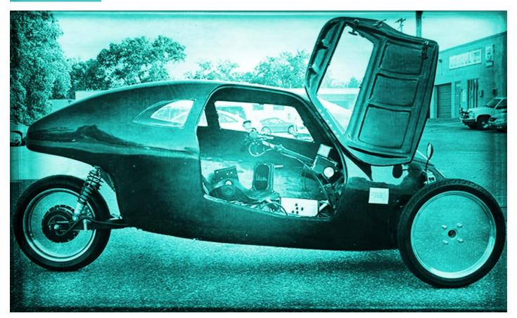
The Racer Cycle is a 3-wheel electric hybrid vehicle which allows cyclists to travel as fast as cars. The flywheel generator multiplies the pedal power of the driver so that the vehicle can hit a top speed of 160 km/h.
