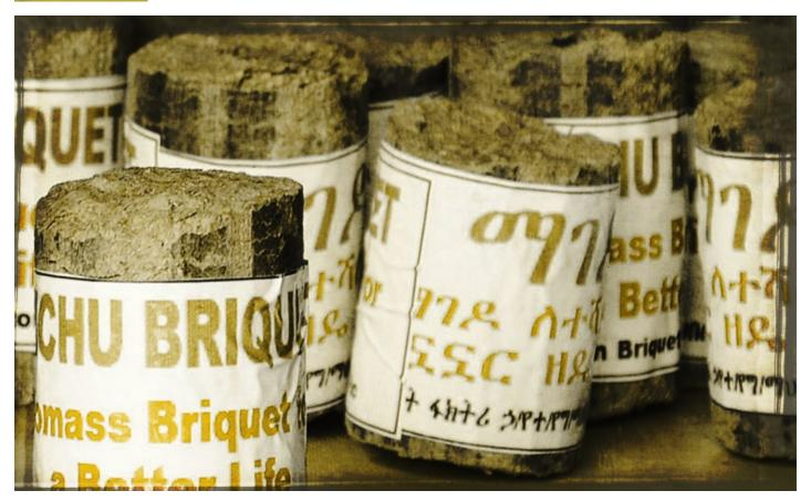
Green coal is made from copmressed loose plants. This way, agricultural byproducts, which otherwise would be rotting waste, are turned into high quality fuel. Green coals are used for cooking or in industrial production.
