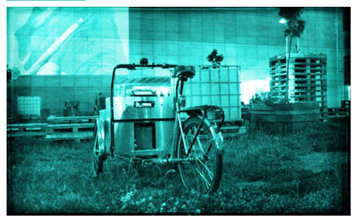
The pedals of the projector bike are used to generate power which is stored in a large battery for a high powered projector and stereo system. The projections can be the size of buildings or as small as a TV set.
