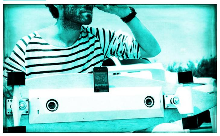
Dutch designer Bjorn van den Hout created the Chargeboard, which is a longboard that charges smartphones. It generates its own electricity through two hidden dynamos, storing it right away into a power box.
