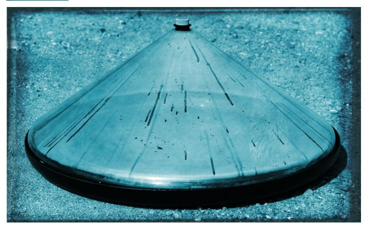
The water cone purification is based on evaporation. It requires sunlight and time. The water cone can purify 1.5 liters of water per day, not only killing all waterborne pathogens but also removing particulates, many chemicals and heavy metals.
