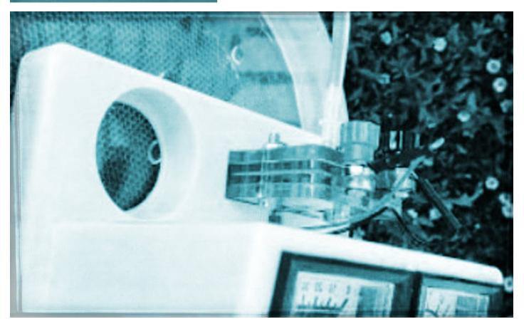
The 17-year-old student Cynthia Sin Nga Lam created the device H2PRO which purifies waste water, while simultaneously generating electricity. The process needs titanium dioxide and light. It is made to be used in developing countries.
