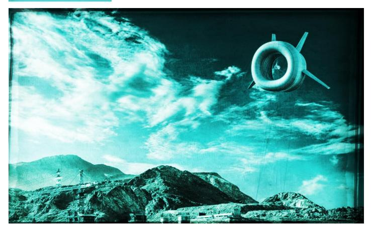
Since winds are much stronger and more consistent at high altitudes, flying wind turbines are more productive than ground-based turbines. In addition, flying wind turbines are less problematic with birds and the surrounding environment.
