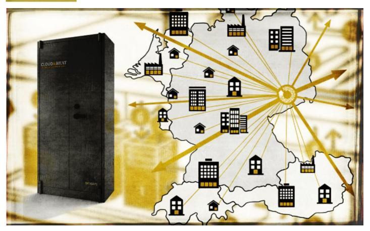
The company Cloud & Heat offers free heating. They place servers in offices where they process cloud data for internet users. Meanwhile, the heat generated by the servers is used to heat the building and water.
