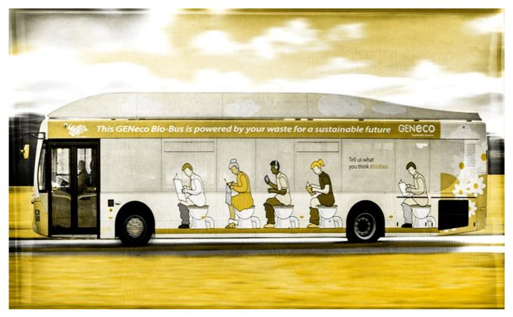
The Bio-Bus runs on gas generated through the treatment of sewage and food waste. It produces fewer emissions than traditional diesel engines and helps to improve urban air quality in Great Britain.
