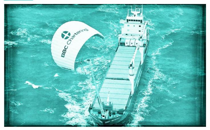
The SkySails system tows the ship using large, dynamically flying towing kites, which generate up to 25 times more energy per square meter than conventional sails propulsion systems.
