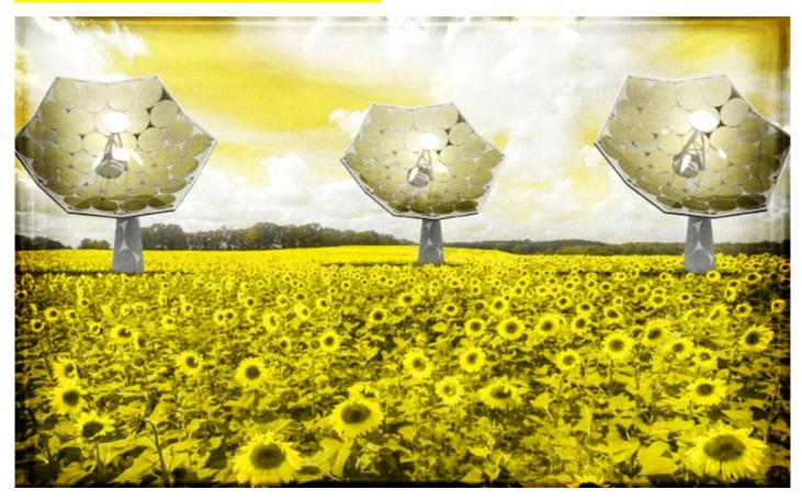
The photovoltaic system can concentrate the sun's radiation 2,000 times. It converts 80 percent into useful energy to generate enough electricity to power several average homes.
